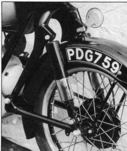
Reynolds-Earles design on the Douglas Dragonfly features separate torque arm
