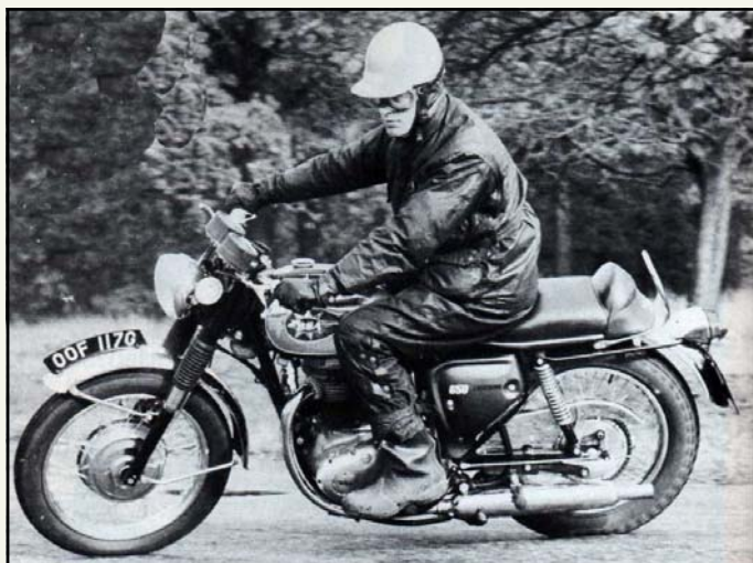
Above: buyers of BSA's unit construction A65 twins benefitted from almost square bore and stroke dimensions of 75 x 74mm, compared to 70 x 84mm for the previous A10 650's
