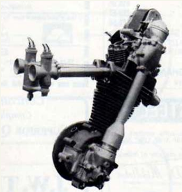
The Beardmore had it all – shaft and bevel camshaft drive, a four-valve head, an outside flywheel and a horizontally split crankcase
