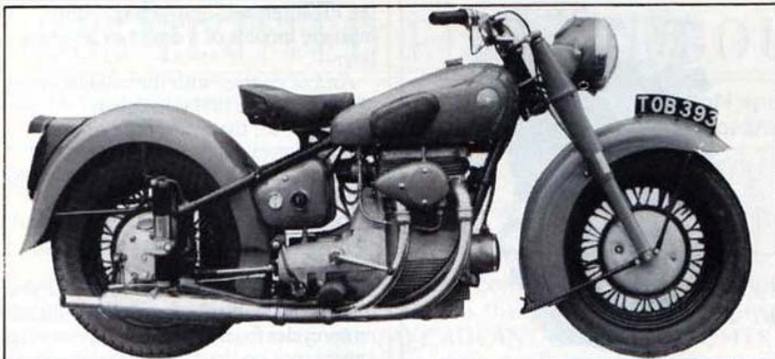
Transmission flaws rather than engine faults marred the postwar sohc Sunbeam twins
