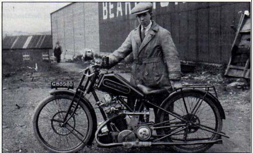
Long induction stubs and a magneto on top of the engine were features of the ill-fated 1924 Beardmore
