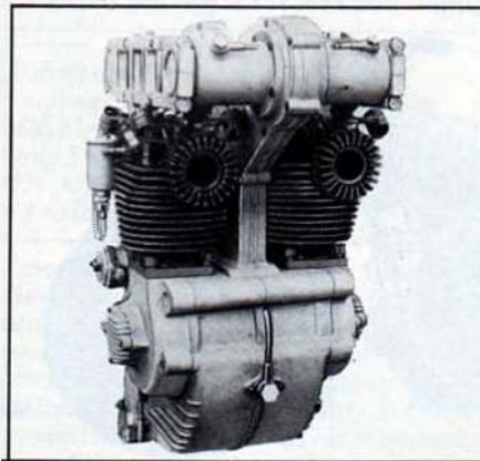
What the British should have made? This 350cc twin with a four-bearing crank and central gear drive to twin overhead camshafts was produced by Italy's Azzariti factory in 1934
