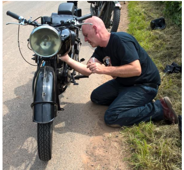
Nick, having a James Herriot moment trying to insert his arm under the fuel tank of the Velo to locate the clutch cable adjuster.
