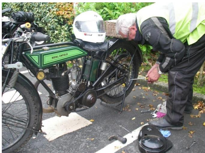
Exhaust repairs needed and Primary Chain adjustments in progress at the lunch stop.
